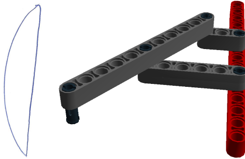
Fig. 3. Chebyshev's \lambda mechanism (1878) and the sextic it draws in one movement. The pen refill should be inserted at the left end of the beam with 11 holes.
